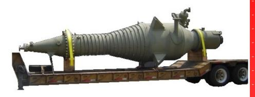
filtration system for process gas and steam, suitable for all applications where working conditions prevent the use of cyclones or bag houses.
